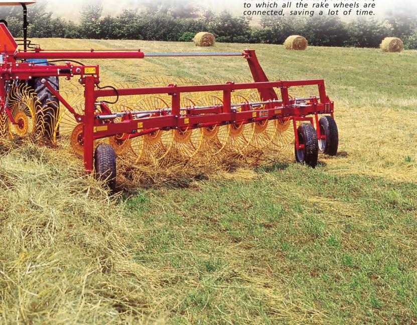
**Single side opening kit** A valve, simple to fit and to handle, can be set so as to choose only one of the wings of the hay rake, the one on the right or on the left, as required, without having to install or remove any parts on the machine. The kit is extremely simple to use, and enables easy overturning of damp swathes or those that have not dried out completely, so as to speed up the drying process.
