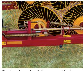
Each rake wheel has an adjustment spring. When the spring is suitably stretched, it ensures that the pressure of the associated rake wheel against the ground is just right, to make sure of excellent raking on any terrain. After this initial adjustment of the individual rake wheels, it is possible to make all the subsequent adjustments effective on the whole wing of the hay rake thanks to a crank, that operates a shaft, to which all the rake wheels are connected, saving a lot of time.
